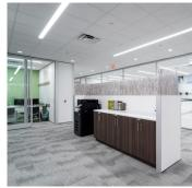
We installed 955+ linear feet of DIRTT manufactured wall systems in and 305 linear feet of DIRTT millwork to reduce initial construction schedule from nine weeks to five.
